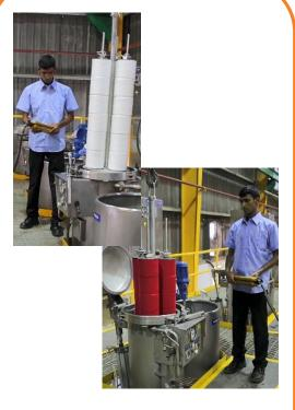
Application of colour through batch processing with dyes and chemicals
