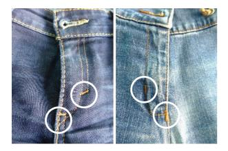
An internal or external bartack must be used to protect the zip from damage caused during special garment processes. The bartacks also protect the zips if the wearer accidentally steps on the garment.
