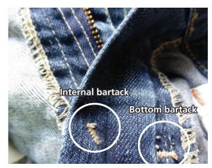
A correctly constructed bartack normally offers 3-4 times higher protection strength than the zip teeth and bottom stop. Single or double lines of stitching do not offer sufficient protection and can break easily during washing or the wearer's use damaging the zip components.
