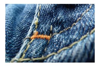
The bartacks prevent damage during the industrial wash (enzyme or stone or bleach washing) process, where loading / forces can be more than 100 times of a domestic washing process or the anticipated loads exerted during the normal wear of the garment.
