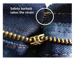
The safety bartack takes the load applied during wearing of the garment, thereby preventing damage to the zip slider, teeth and bottom stop.
