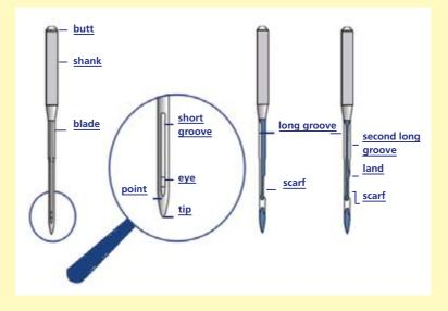
A needle has various parts to execute different functions during the sewing operation as follows:
