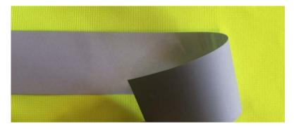
3. <u>Step 3</u>: After lamination, allow the application to cool to room temperature and carefully remove the liner on the reflective side. Allow a long cooling temperature of up to one hour. To remove the liner, lift the film from one corner and pull it gently with a single motion while holding the substrate flat.
