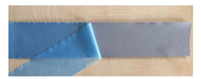
2. <u>Step 2</u>: Place the heat transfer on the substrate surface with the adhesive side down facing the substrate. For heat press, the temperature and pressure should be even on the tape. Use a press cloth, a siliconized slip-sheet or a Teflon heat pressing sheet to cover the heat transfer and the fabric during lamination to avoid any surface damage. For two times pressing, allow the fabric to cool down after first pressing and press again using the same lamination conditions.
