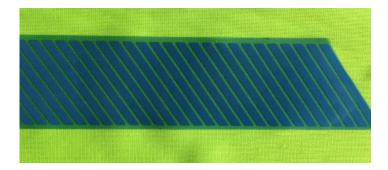
3. <u>Step 3</u>: After lamination, allow the application to cool to room temperature and carefully remove the liner on the reflective side. Allow a long cooling temperature of up to one hour. To remove the liner, lift the film from one corner and pull it gently with a single motion while holding the substrate flat.
