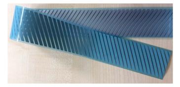
2. <u>Step 2</u>: Place the heat transfer on the substrate surface with the adhesive side down facing the substrate. For heat press, the temperature and pressure should be even on the tape. Use a press cloth, a siliconized slip-sheet or a Teflon heat pressing sheet to cover the heat transfer and the fabric during lamination to avoid any surface damage. For two times pressing, allow the fabric to cool down after first pressing and press again using the same lamination conditions.
