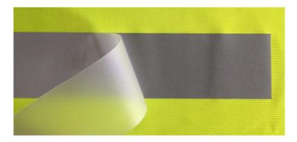
To ensure adequate adhesion to the substrate for the lifetime of the finished product, it is strongly recommended to test the application under the intended care instructions for the finished product prior to bulk production. Follow the care instructions from our product data sheet.
