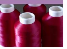
Gral<sup>™</sup> is a lubricated polyester thread made from pre-stablised high tenacity continuous filament polyester which is excellent for all types of leather and offers good abrasion resistance. The soft finish with superior low friction lubrication reduces the effects of needle heat and abrasion. The higher breaking strength and optimum stretch characteristics produces attractive, fine seams.
