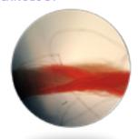
YARN ENCAPSULATION IN HELICAL CORE AND COVER CONSTRUCTION
